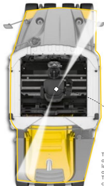
The driver sits on the left or right of the platform while compacting, looking past the engine cover or water tank respectively. This means that he has the construction site in view at all times.
