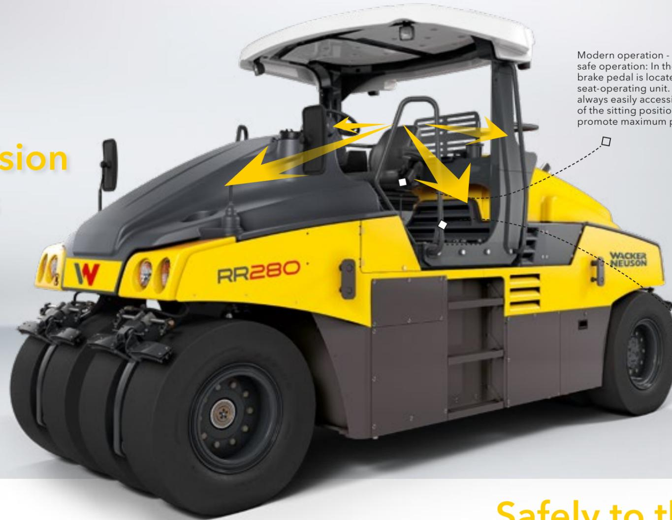
Modern operation - safe operation: In the RR, the brake pedal is located on the seat-operating unit. As a result, it is always easily accessible, regardless of the sitting position. This helps to promote maximum possible safety.
