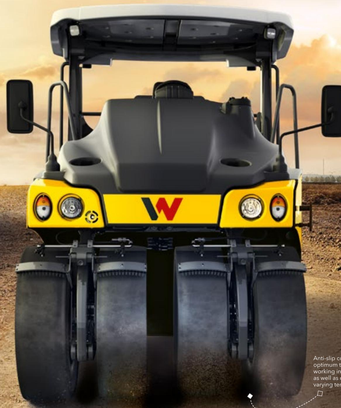
Anti-slip control ensures optimum traction when working in uneven terrain as well as on surfaces with varying temperatures.
