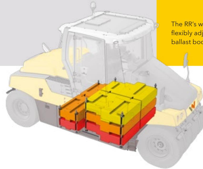
The RR's weight can be simply and flexibly adjusted using prefabricated ballast bodies.
